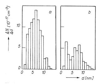
Fig.1. Size distribution of silver particles for sprayed layers treated in a redox buffer solution with  $\Delta E = 0.068$  V, treatment time 0 s (a), 30 s (b).
