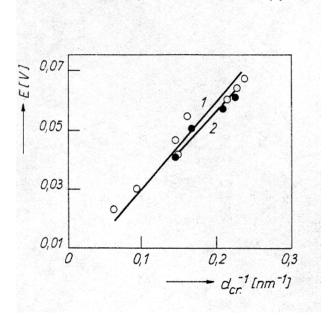
Fig.3. The value of critical-size silver particle inverse diameter vs. the overpotential.
