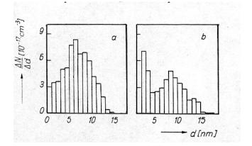
Fig.2. Size distribution of silver particles coated with gelatin after treatment in redox buffer solution with  $\Delta E = 0.058$  V, treatment time 0 s (a) and 60 s (b).
